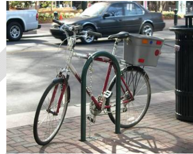
Example of an “Inverted U” bicycle rack. This rack will hold two bikes.
