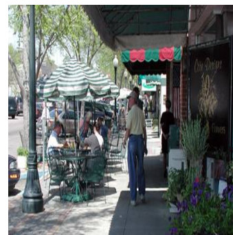
Typical sidewalks in mixed-use commercial areas should be 12-16 feet wide to encourage outdoor seating while providing adequate passing clearance
